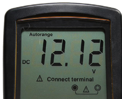
Test Connection between Clamp 1 & Clamp 2 of 12V Cell
