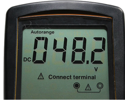
Test Connection between Clamp 1 & Clamp 5 of 12V Cells
