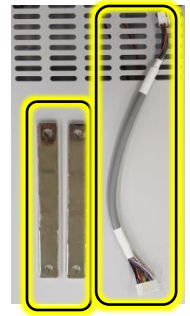
Figure 4c. Bus Bars and Communication Cable
