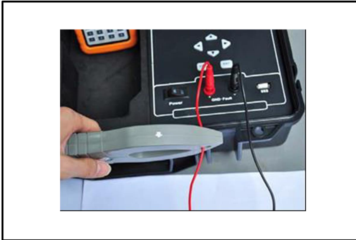
Figure 1-1 Current Clamp Position for Reference Calibration
