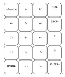
In keyboard, number 0~9 can be used to select menu operation or parameter setting. <↑>: Upward button, each pressing can make cursor moving upper one grid, also can be used to page up on the screen.
