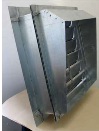
Louver set up for Supply Fan
