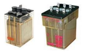
**Large VLA single and multi-cell units.** Usually 2 to 8 Volt units, ranging up to 4000 Ah at the 8 hour rate and up to 4000 Watts-per-cell at the 15 minute rate. Some examples are shown below. Designated life 20 years. Actual life with UPS applications, 12 years. With Telecom and Utility applications, 15 to 20 years.
