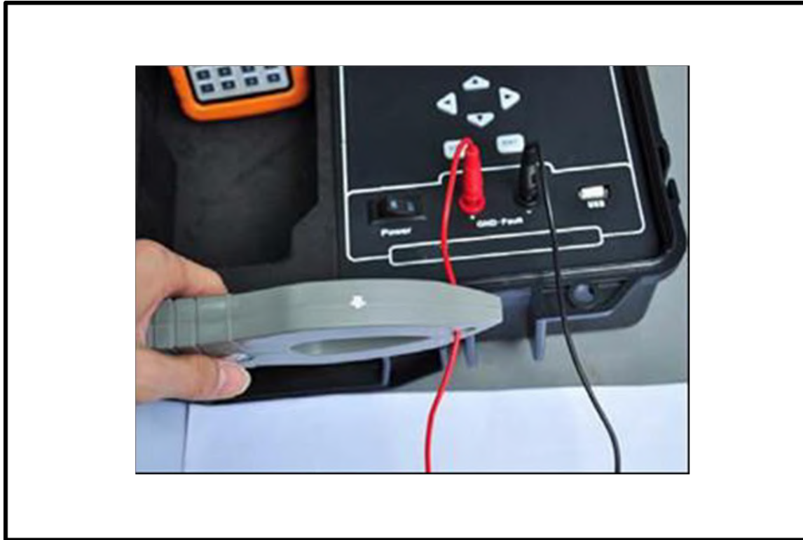
Figure 4-9 Current Clamp Position for Reference Calibration
