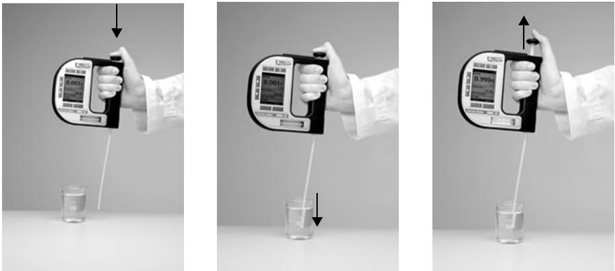
Fig. 10 - 1 Filling sample using the filling tube
