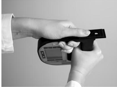
*Fig. 12 - 3 Removing the pump lock*
