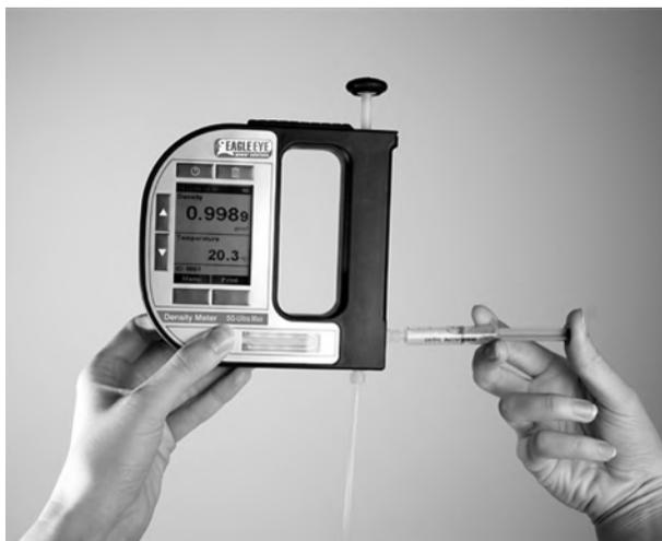
Fig. 10 - 2 Filling sample using the plastic syringe
