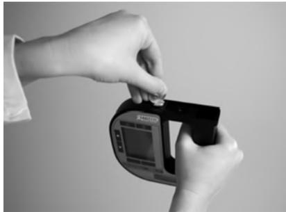
*Fig. 12 - 4 Opening the battery cover*
