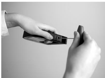
*Fig. 12 - 2 Removing the pump lock screw*
