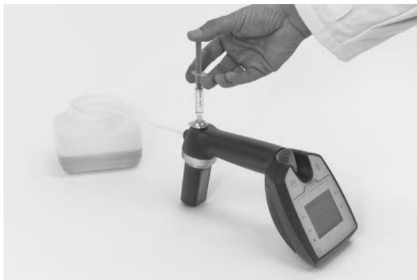
Fig. 12-2: Filling sample using a syringe
