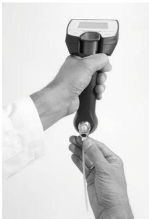
*Fig. 6-1: Connecting the filling tube*
