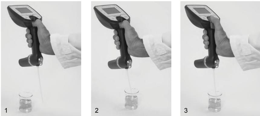
*Fig. 12-1: Filling sample using the filling tube*
