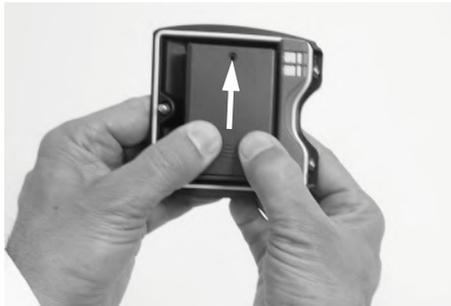
*Fig. 15-2: Removing the battery compartment*
