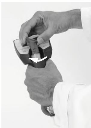
*Fig. 14-3: Remounting the pump*
