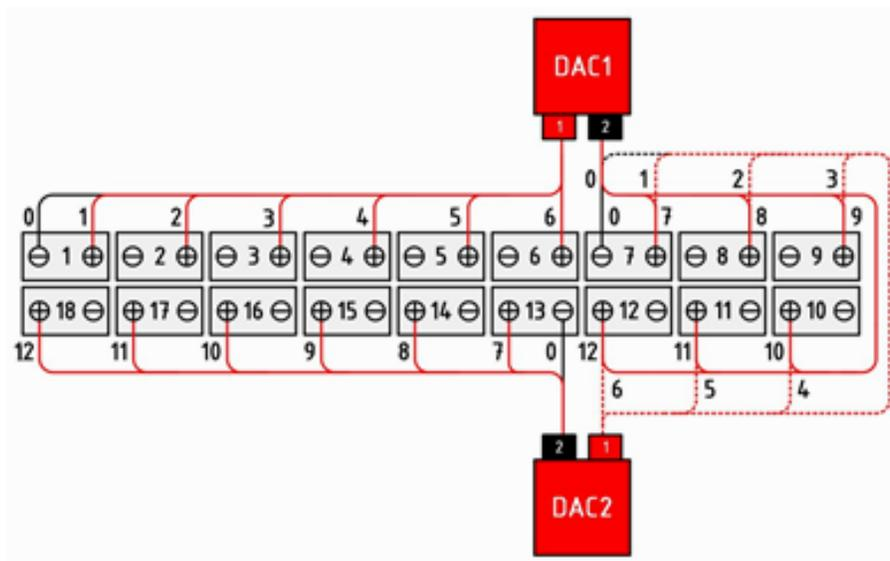
**Notice:** With DAC #2; the #12 lead is connected to the most positive terminal and the user has worked backwards, eventually overlapping several leads of DAC #1.
