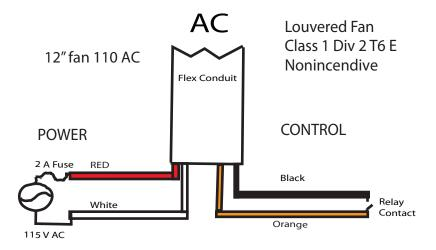
The flexible shielded electrical conduit contains four wires. Red(+) and White(-) are for connection to AC power. See the data plate on the fan for the appropriate voltage. The other two wires are Black and Orange and connect to a normally open switch or relay contacts. Contact closure activates fan.
