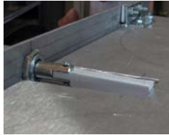
Positive shut off doors closed
