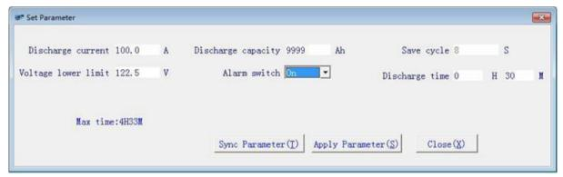
If you want to get the present parameters, click [Sync Parameter], the parameters in the software can be replaced by that of lower position computer.
