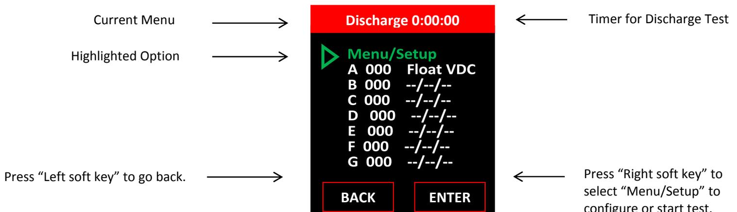
**Note: User must record float readings before being able to start Discharge Test!!!**
