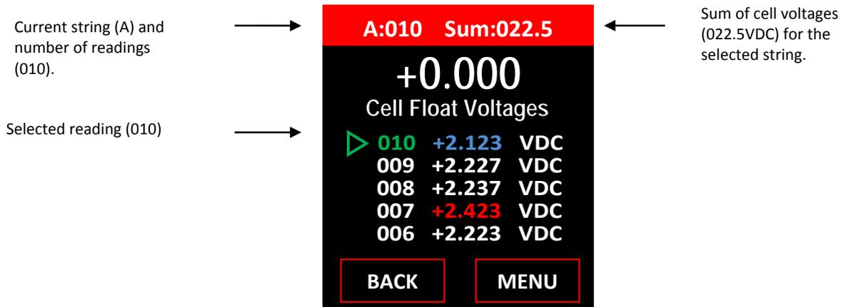
For example, after taking 10 cell float voltage readings of average ~ 2.25 the DLV-Pro display should match the above.
