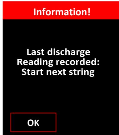
The User can now start recording the **second set** of discharge cell readings in string C. This process is repeated until the discharge test is completed or all the available Strings (B through K) have been used.
