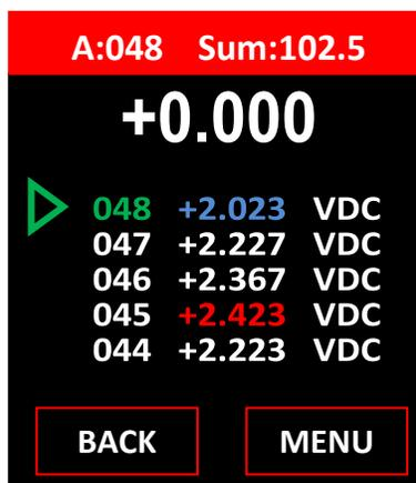
**6.0** When a reading is deleted **ALL** readings in memory locations **above** the deleted cells are moved **down** (1) location.
