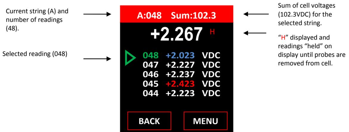
(vi) Remove the voltage probes from the cell terminals.
