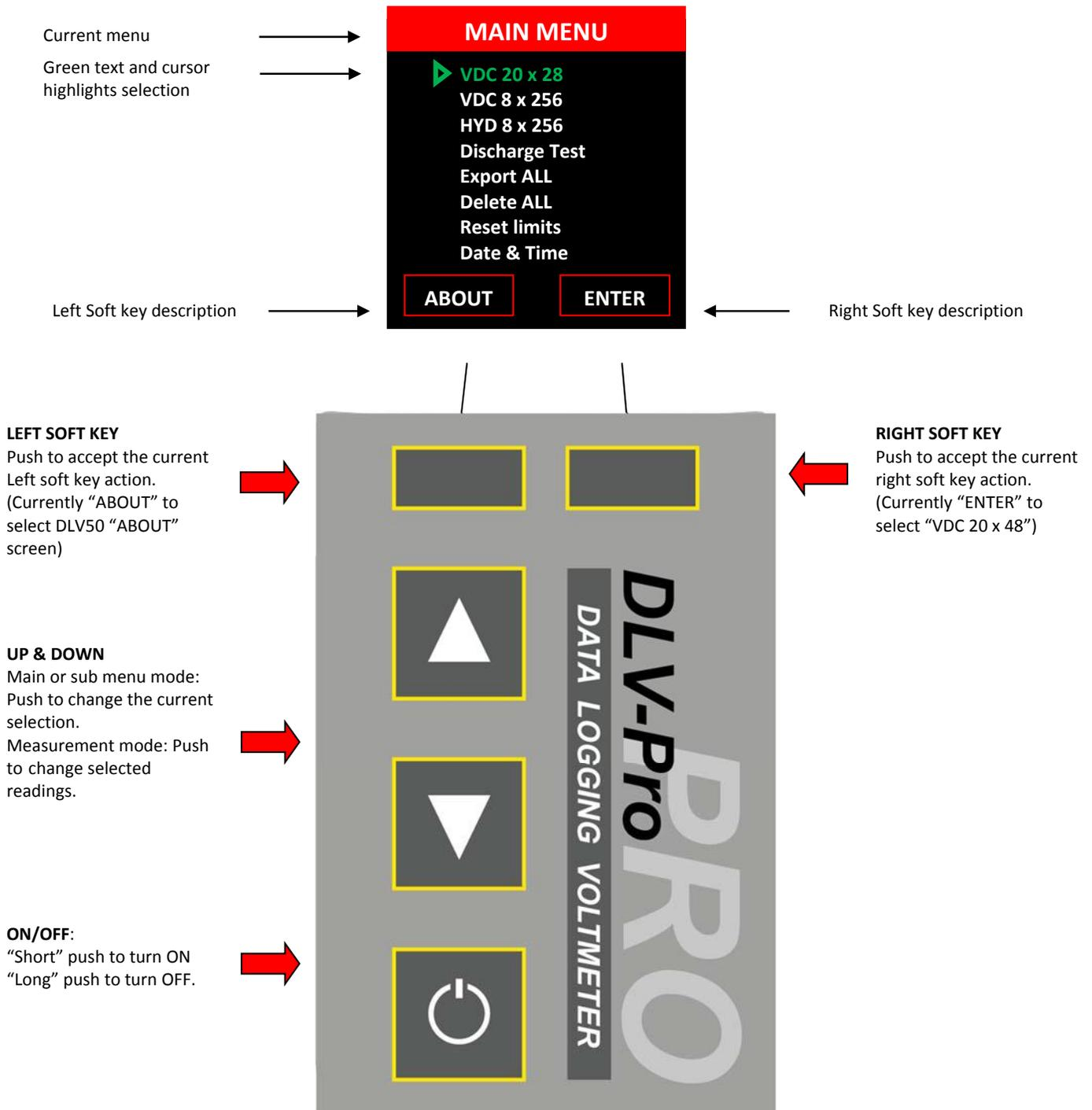
Regardless of DLV-Pro status, repeatedly pressing the left soft key will return the unit to the Main Menu (unless the DLV-Pro is connected to a PC via USB).
