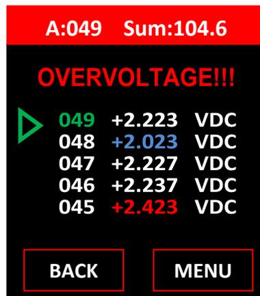
This warning is removed as soon as the probes are disconnected from the high voltage source.
