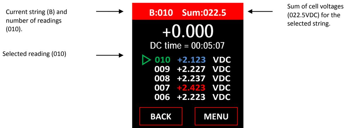
For example, after taking the first (10) cell discharge voltage readings of average ~ 2.25, the DLV50 display should match the above.
