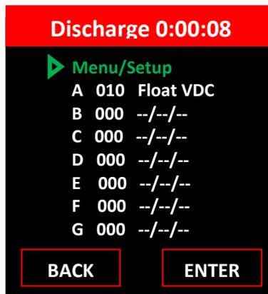
After the discharge test timer is started the elapsed time is shown.
