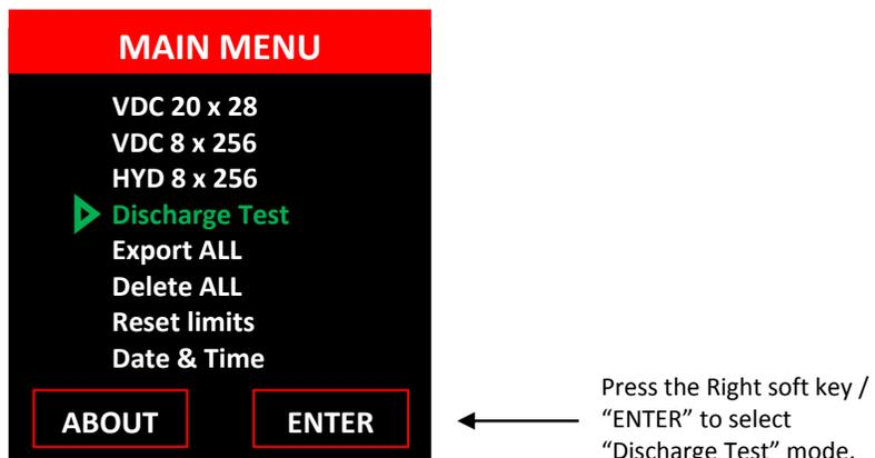
The DLV-Pro will change to “Discharge Test Mode” and display current mode information:
