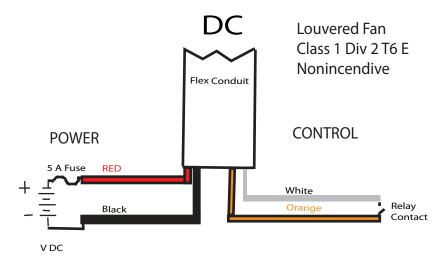
The flexible shielded electrical conduit contains four wires. Red(+) and Black(-) are for connection to DC power. See the data plate on the fan for the appropriate voltage. The other two wires are White and Orange and connect to a normally open switch or relay contacts. Contact closure activates fan.
