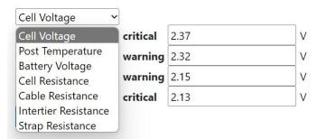
All **critical** alarm limits will trigger relay 1 on the monitor and also illuminate the "Battery Alarm" LED on the monitor red.
