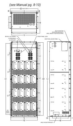
**16-Slot Chassis** Dimensions & Weight 18.93 x 51.25 x 14.47 in. (481 x 1302 x 325 mm) 296 lbs. (134 kg) 200 lbs. (90 kg) unloaded
